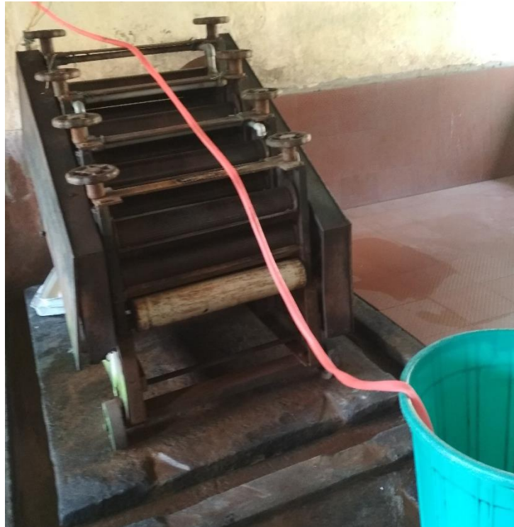
Rubber Sheet Manufacturing Machine in the RPS of Purana Senapati Para of Gomati District
