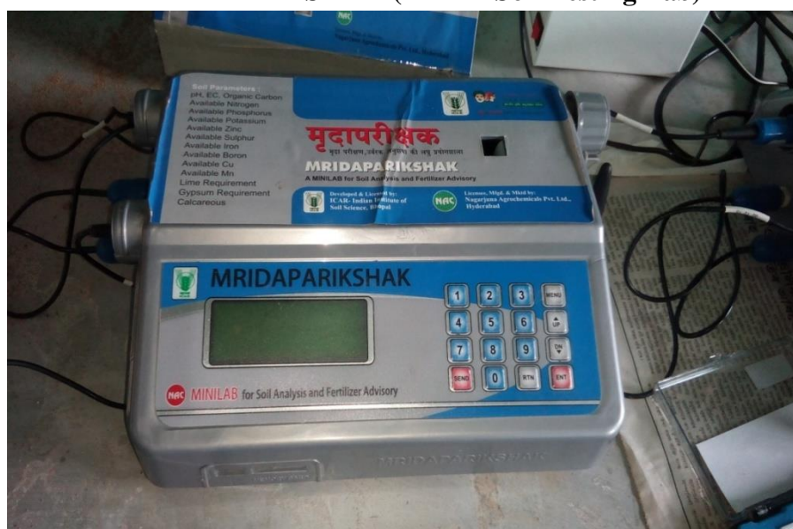
Image – 1.2 MRIDA PARIKSHAK (A Mini Soil Testing Lab)
